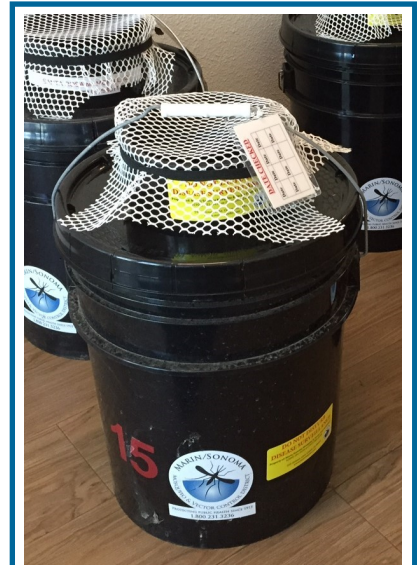
Autocidal Gravid Ovitrap (AGO) The AGO trap is deployed to detect invasive Aedes adults female mosquitoes that are looking for a place to lay their eggs.
